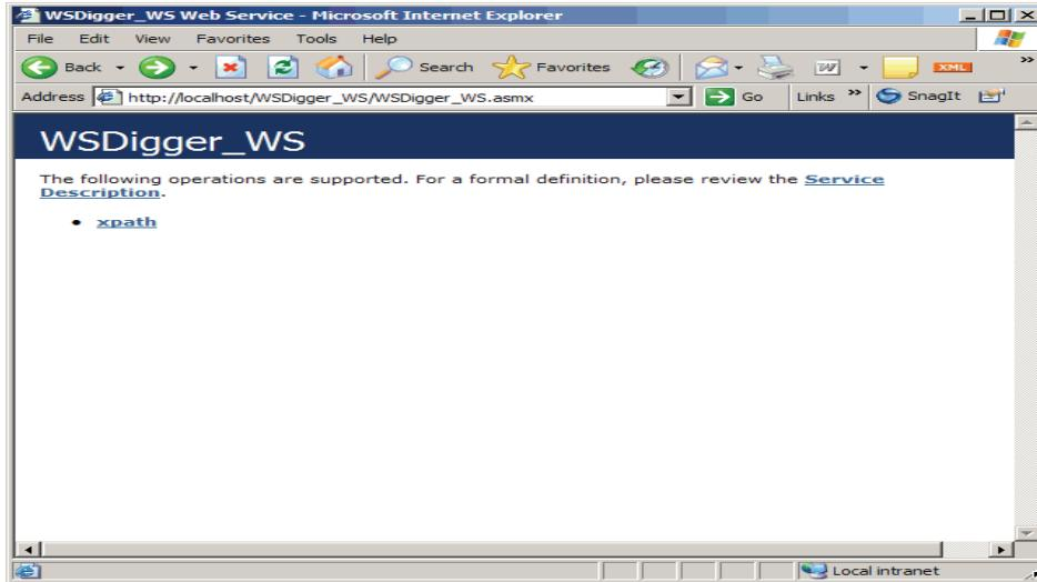
Launch WSDigger and hit next to get to the WSDL screen. Enter [http://localhost/WSDigger\\_WS/WSDigger\\_WS.asmx?wsdl](http://localhost/WSDigger_WS/WSDigger_WS.asmx?wsdl) in the WSDL textbox and hit 'Get Methods'. The result displays methods enumerated.
