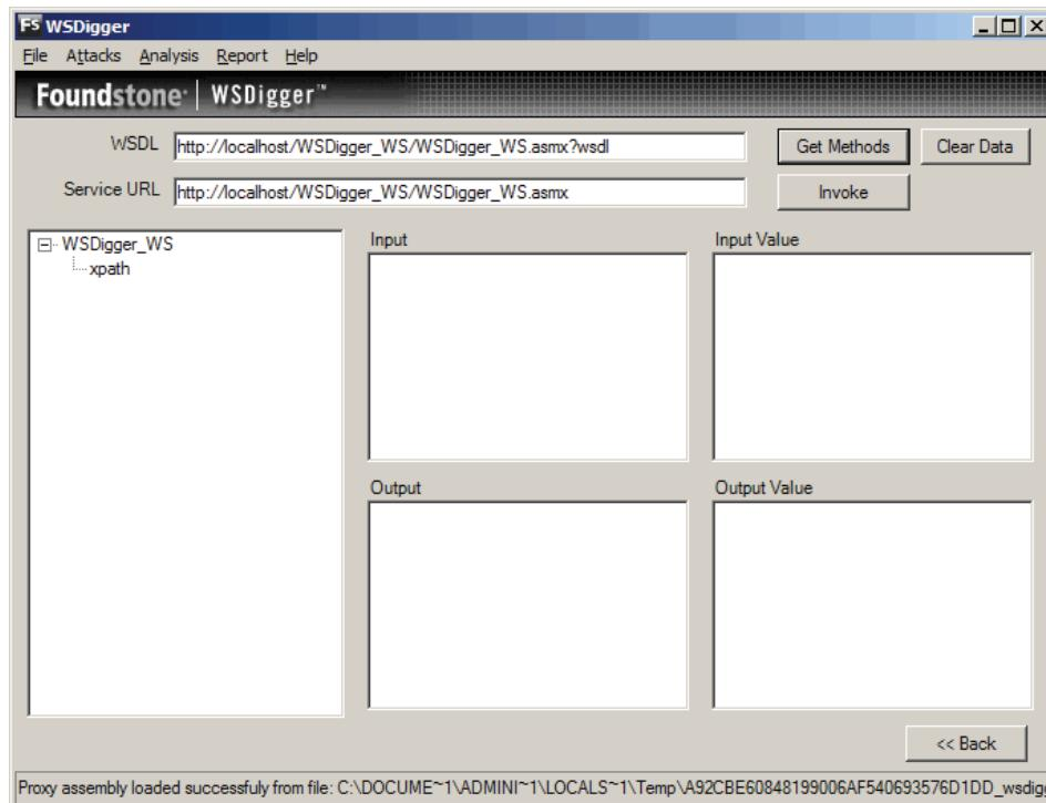
Browse to Attack ->Select Attack Types. Select all 3 attack plug-in and hit enter. Once the tool is finished, browse to Report -> Generate Report. The report is generated and displayed in the default browser. The web service is vulnerable to XPATH Injection and dumps the complete database.
